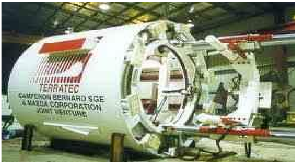
Slurry Shield TBM
