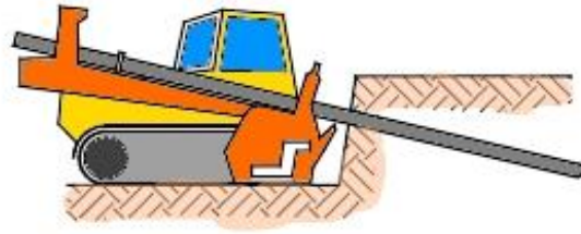
STEP 2. DRILL NAIL HOLE
