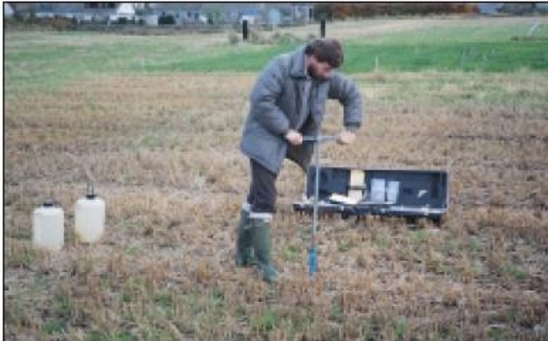
1 Auger and prepare hole
