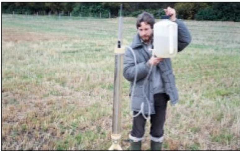
2 Install Permeameter and fill with water
