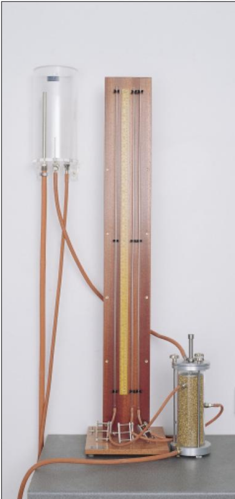
Constant Head Cell with manometer tubes and Constant Level Tank
