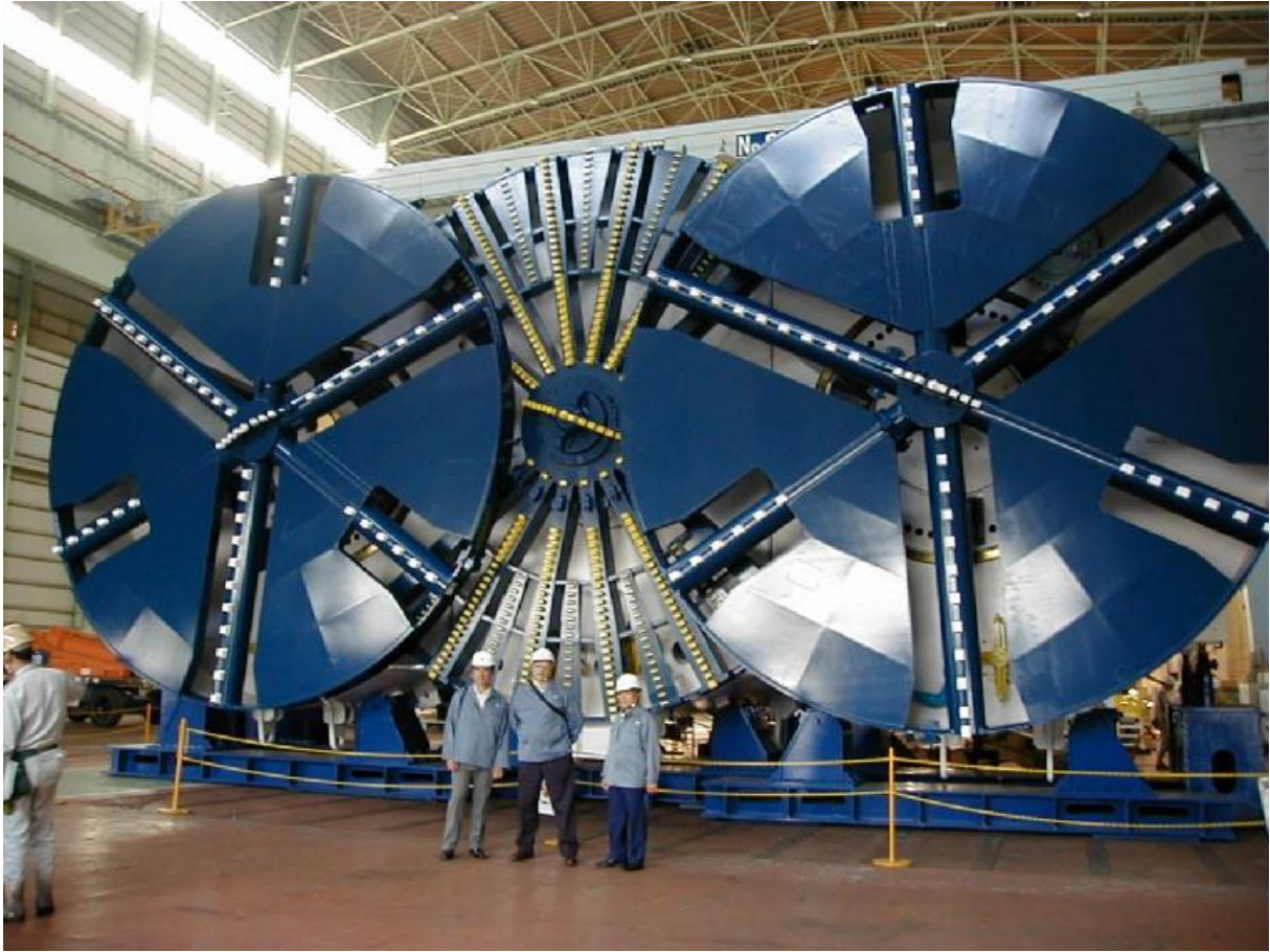
Tunnel Boring Machine
