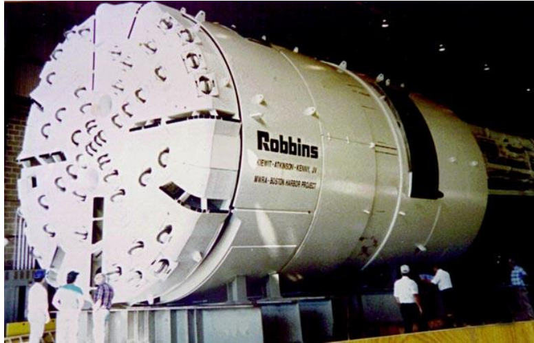
Tunnel Boring Machine (TBM)
