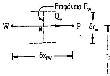
$$f_w \equiv \frac{\exp(P_{ew})}{\exp(P_{ew}) - 1} \quad P_{ew} \equiv \frac{r_w U_w dX_{pw}}{\Gamma_w} \text{ (αριθμός Peclet)}$$
