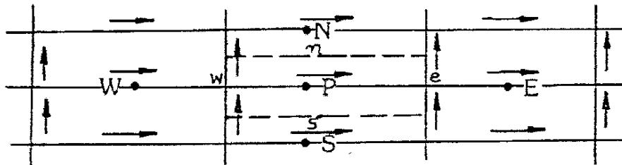
$$a_w = p_w U_w E_{ew} f_w, \quad E_{ew} = r_p \delta r_{ns}, \quad f_w = f_{\text{Hybrid-Difference}}(R_{ew})$$
