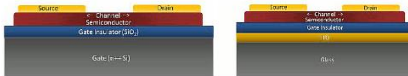
Schematic of bottom gate, top contact OFETs using Ossila's source-drain evaporation stack and Si/SiO 2 substrates (top) and ITO substrates (bottom).
