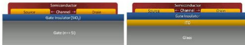
Schematic of bottom gate, bottom contact OFETs using Ossila's source-drain evaporation stack and Si/SiO 2 substrates (top) and ITO substrates (bottom).
